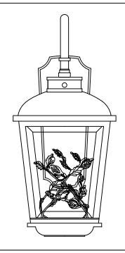
To prevent water intrusion, caulk around back-plate where fixture meets the wall using outdoor silicone sealant. Leave a small gap at the bottom to allow moisture to exit.
